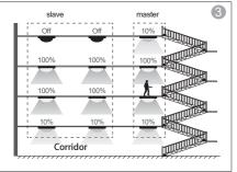
The person walks to the 3rd floor, the 3rd sensor highbay switches the light on 100%. All slaves on the 3rd floor turn the light on and the Sensor highbay on the 4th floor switches onat stand-by level. Meanwhile, the lights on the 1st floor are dimmed to stand-by level after hold-time.
