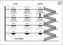
The person walks to the 4th floor, the 4th sensor highbay switches the light on at 100%. All slaves on the 4th floor turn the light on Meanwhile, all sensors on the 1st floor turn the light off after stand-by period, and all lights on the 2nd floor dim to stand-by level after hold-time.
